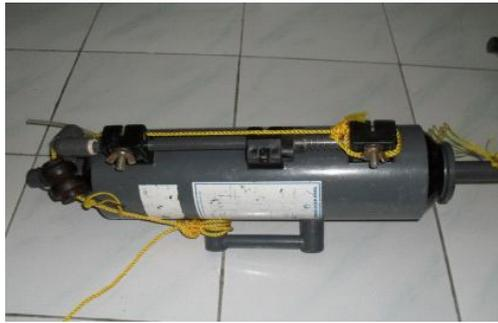
Gambar 2. *Kemmerer water sampler*.
