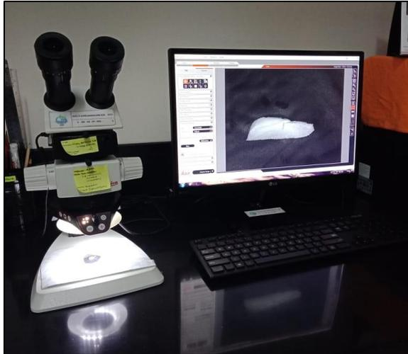
**Gambar 4.3.** Proses pengambilan gambar *otolith* tuna sirip kuning.
