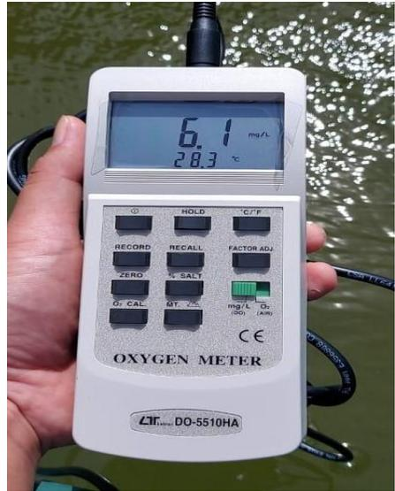
Gambar 5. Alat pengukur DO & Suhu
