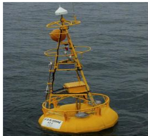
Gambar 2.11.7 Wave Recorder jenis AWAC, 2,11.8 Buoy wave recorder. Sumber : BMKG, Maritim.Bitung.2017
