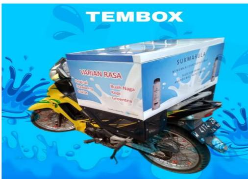
**Gambar 66. Tembox (Thermoelectric cool box)**
