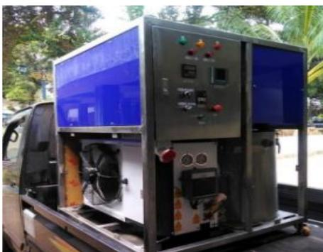
**Gambar 63. Mesin slurry ice**
