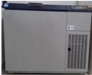
Gambar 16. Alat refrigerator -70°C.
