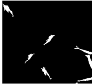
Figure 6. Differentiation of the results of the thresholding process T=175 in distinguishing between objects that are vannamei shrimp and non-vannamei shrimp objects.
